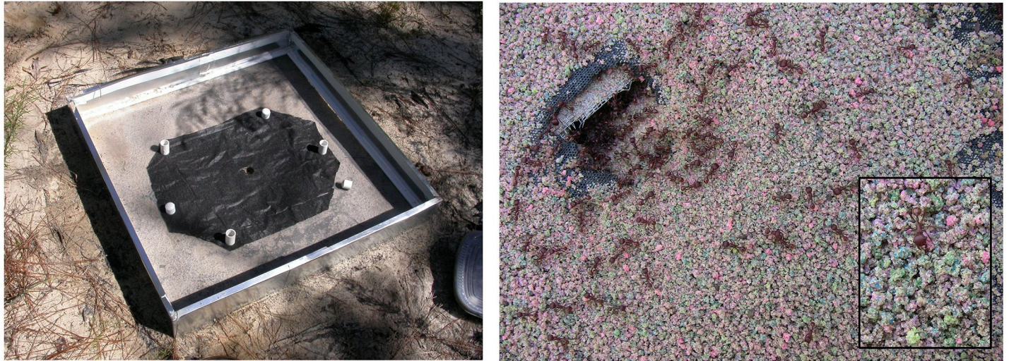
Fig 2. A. The screen-bottom box into which the P. badius colony was released to dig a nest through a central hole in the screen into the "layer cake" below. The black weed mat allowed the easy collection of the sand the workers brought to the surface every day. B. An example of the sand brought up to the surface by the ants during one day. The inset shows a detail of colored sand pellets dropped by the ants.
